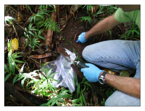
Photograph F-46: Incremental Soil Sampling at SU BKG-01, Collection of Single Increment.
