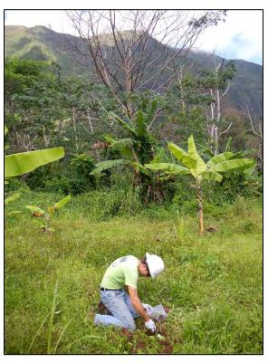
Photograph F-50: Incremental Soil Sampling at SU MVIA-03. Direction Facing: North
