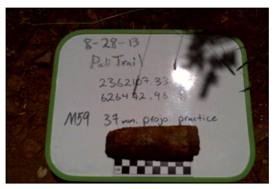
Photograph F-23: Munitions Debris Located on Pali Trail.
