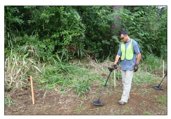
Photograph F-3: UXO Sweep Team Member Performing Instrument Check at Instrument Testing Strip.
